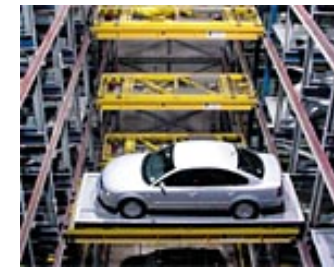
Forget parallel parking | At the Hoboken Garden Street Garage, automated carriers store and retrieve cars in double bays on both sides of the center row.
