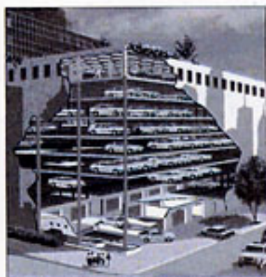
Cutaway of complete Robotic Parking structure
