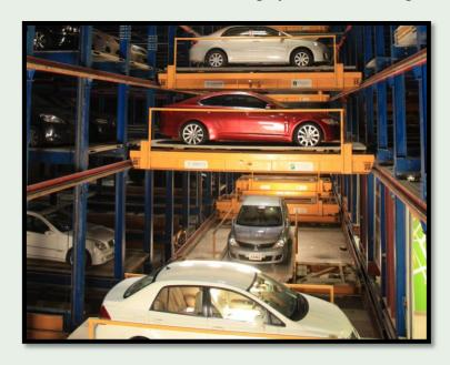
Robotic Parking Systems Inc. has more than 15 years of experience designing, building and operating our Robotic Parking garages. The entire system was designed from the very beginning to overcome any possible machine failure so that <u>cars can be retrieved no matter what</u>. This design point is represented in the system architecture, its redundancies and flexibilities.
