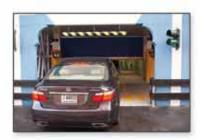
2. Drive into one of the convenient parking terminals indicated by a green light. Multiple automatic sensors ensure that the car is properly positioned for parking. Robotic Parking Systems offer more safety and security.
