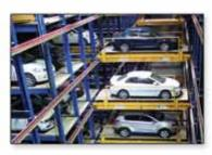
5. Robotic Parking Systems does the rest. The car is picked up by the computerized machinery and lifts that safely place it inside the building on a shelving system. The Ibn Battuta Gate facility handles 250 cars per hour with up to 32 cars in motion at any time.
