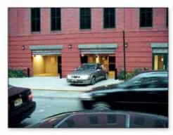
Designed, implemented and operated the 314 space automated parking facility. The Robotic Parking System was operated 24 / 7 for four years with 99.9% uptime over 750,000 vehicle transactions and approximately 34,000 hours.
