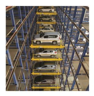
The first phase of this evolution was to create a more efficient, safe, and effective parking solution, handling more cars quickly on a smaller urban footprint. As technology and the diverse number of transportation options have appeared over the last 25 years, Robotic Parking Systems has grown and expanded its offerings. This new strategy embraces the concept of mobility as a service and transforming parking structures into the hub of an integrated Smart City approach.
