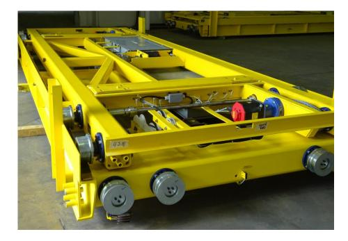
The Robotic Parking System utilizes off-the-shelf, high-quality components with L10 lifetimes of 40,000 hours or above. Electro-mechanical components are used to avoid hydraulic or pneumatic equipment that involves high maintenance.
