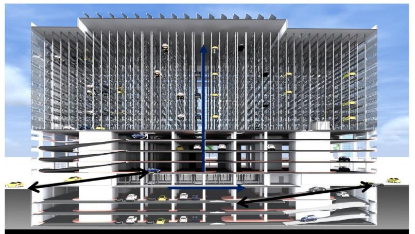
Concrete Ramp = 684 spaces Robotic Parking = 2314 spaces Footprint is 328 ft by 168 ft. Conventional parking is 7 levels in a height of 97.44 ft. Robotic parking is 11 levels in a height of 115 ft. Automated parking provides 3.5 times the number of parking spaces within a similar volume.
